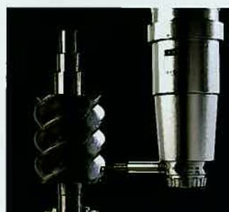
CHECK WITH THREE DIMENSION MEASURING MACHINE
